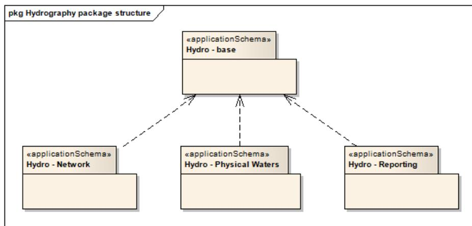
**Figure 2 - Package structure of the Hydrography application schemas**
