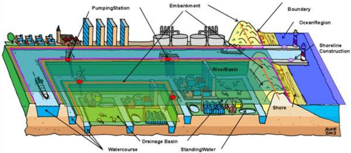
**Figure 33 –Modelling of a polder and associated physical waters / related objects**
