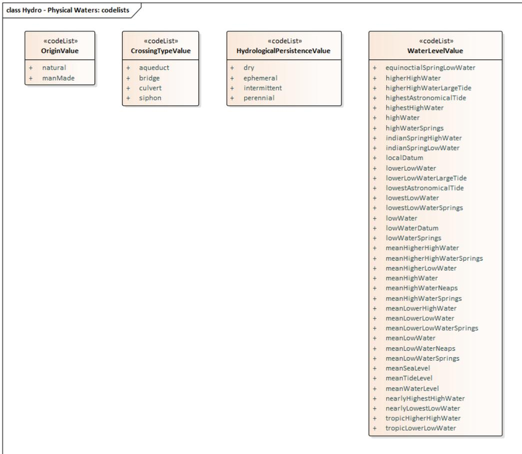
Figure 17 – UML class diagram: 'Physical Waters' code lists
