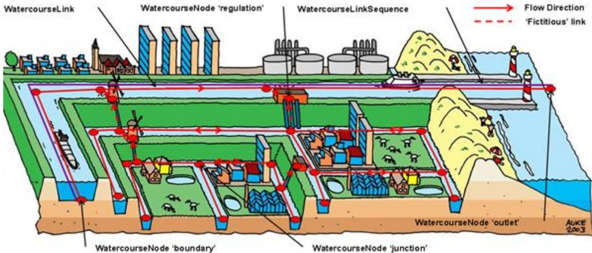
Figure 40 – Network elements in a polder situation
