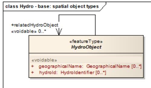
**Figure 4 – UML class diagram: Overview of the 'Hydro – base' application schema**
